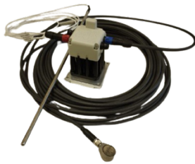
Harvestree fitted with a vibration sensor and an external Pt1000 probe
